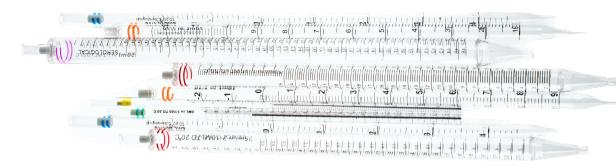
The serological pipettes by MOLEQULE-ON are sterile, individually wrapped and non-pyrogenic. They have both descending & ascending black graduations marks. Top grade resins reduces liquid binding and improves sampling accuracy. Filter plug prevents the liquid from entering pipetting device and their capacity calibration rate is  $\pm 2\%$ . They are available in six volumes.
