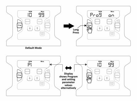
Press the "Program" button to select any program from "P1 to P9". Programs can also be selected by pressing "increment or decrement" button. Once the desired program is selected, press the "speed button" to select and set speed value. Press "Time" to select and set time value.
