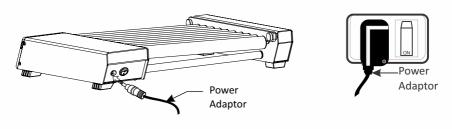
After connecting the power adaptor to back side of device, switch the main power supply to "ON" & then switch the device on from rear. Make sure that tubes are loaded properly before use. Do not start the device if the hinge is open.
