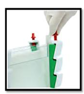
Insert a gel cassette into each side of the inner buffer chamber in the PAGE insert, and begin tightening the vertical screw-pins until the gel clamps glide out of the resting slots and fix firmly against the glass plates pushing them upright.
