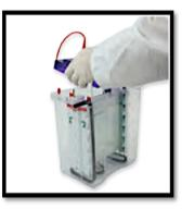
Replace the lid, connect to the power supply and run.
