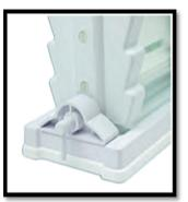
Check the bottom of the glass plates to ensure that they are flush together,
