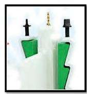
Loosen the vertical screw pins in the PAGE insert to release the locking mechanism, allowing the gel clamps to sit in the resting slots.
