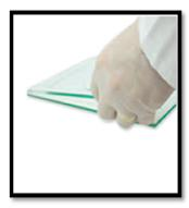
Assemble each gel cassette on a flat level surface, by placing the plain glass plate down with the spacers facing upwards followed by the notched glass plate.
