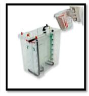
Transfer the PAGE insert to gel the tank. Fill the inner and outer buffer chambers before loading samples
