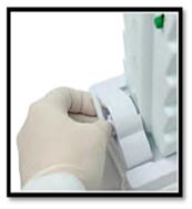
Insert cams and turn until tightened, drawing the PAGE insert onto the casting to form a leakproof seal.
